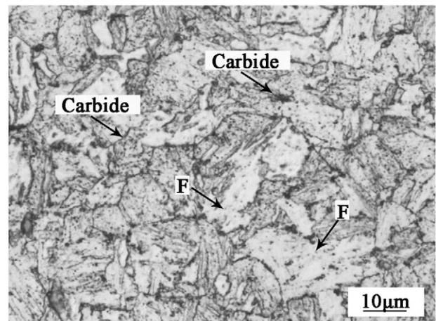
Fig. 2. Microstructure of E550 steel under optical microscope.
