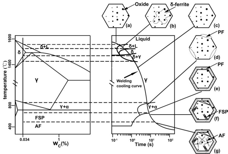
Fig. 1. Schematic illustration of HSAL weld metal phase transformation at continuing cooling condition. Note: AF: acicular ferrite; PF: proeutectoid ferrite; FSP: ferrite side plate.
