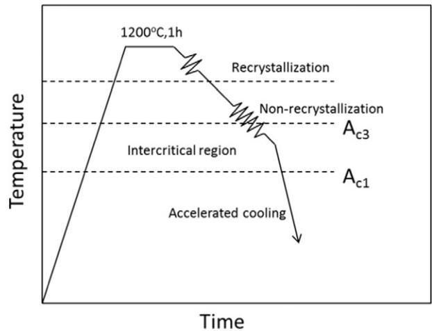
Fig. 1. Schematic diagram of thermo-mechanical processing schedule.
