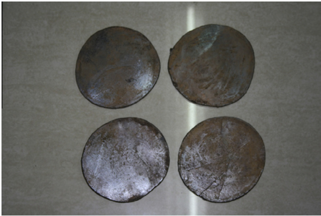
Fig. 1. As forged pancakes (diameter: 130 mm, thickness: 7 mm) of some selected titanium alloys.
