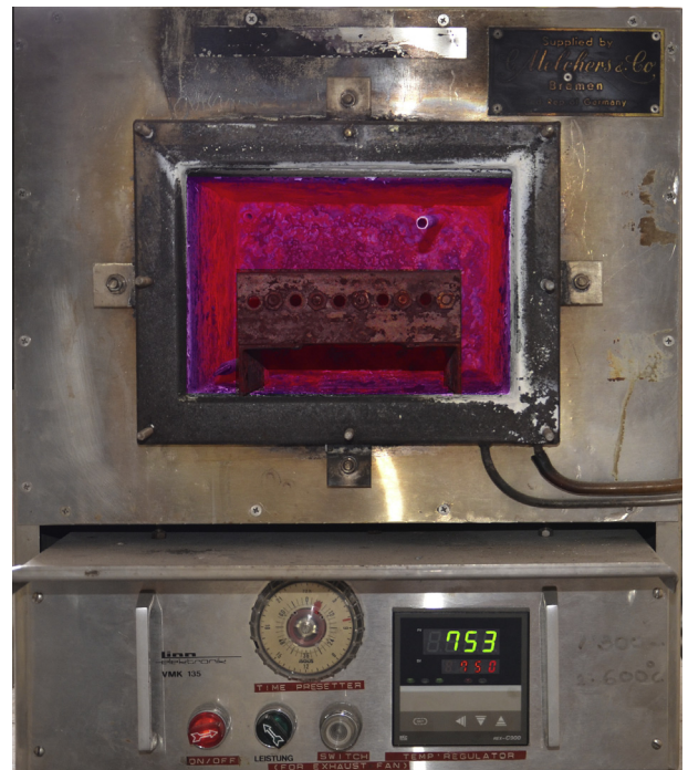
Fig. 2. Fixture in the furnace.
