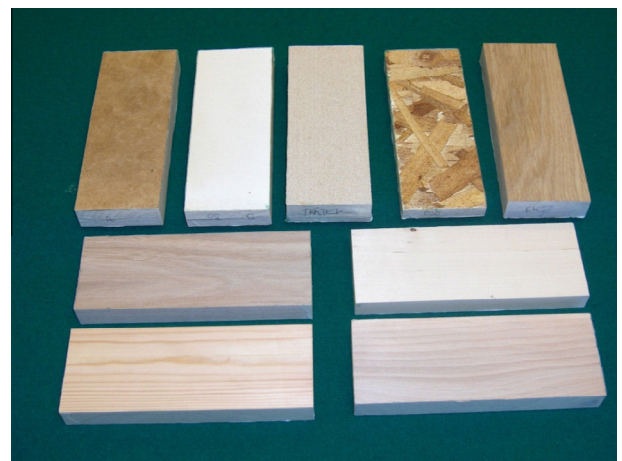
Fig. 1. Wood and composites used in the tactile study. Top row from left: Comp A 60% unbleached softwood craft pulp in PLA, Comp B 60% fully bleached birch craft pulp in PLA. Comp C Wood polymer composite, Extruded, wood fibers 50% in PP, OSB, Oak. Second row from the left: Elm and birch. Bottom row from the left: Pine and Ash.
