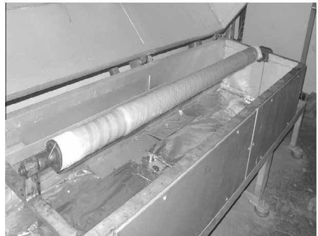
Fig. 2. Composite tube inside oven for cure.
