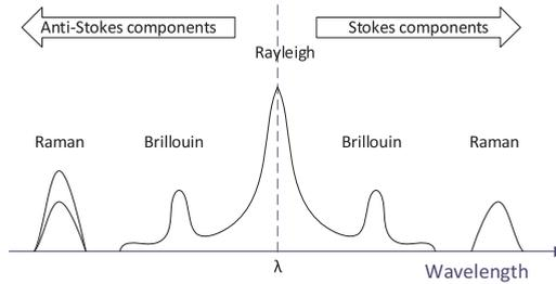
Fig. 1. Scattered light spectrum diagram.
