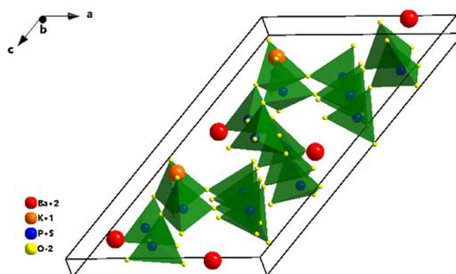
Fig. 1. The schematic views of  $\text{KBa}_2(\text{PO}_3)_5$  crystal structure.
