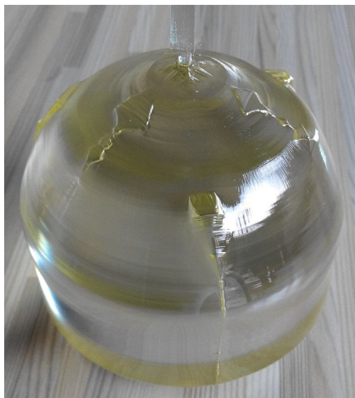
Fig. 1. LiNbO 3 crystal was grown by the Czochralski method.
