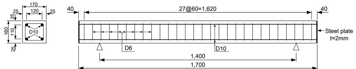
Fig.1. RC beam detail.
