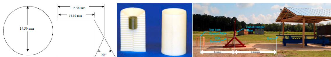
Fig. 1. NATO standard fragment (left), typical sabot (center), and 40mm smoothbore gun (right)
