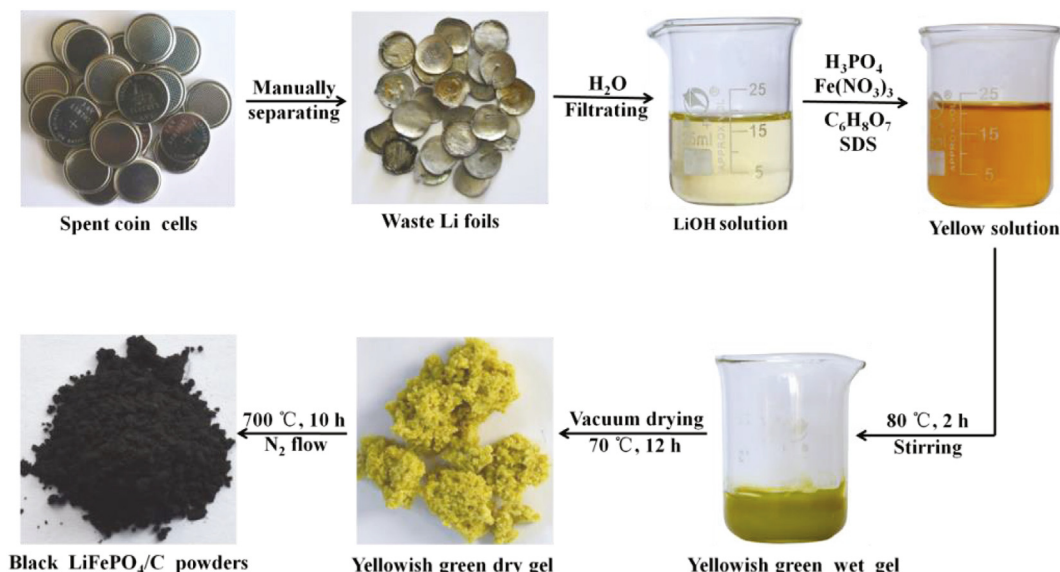
Fig. 2. Recycled procedures of waste Li foils from spent Li-foil-based coin cells.
