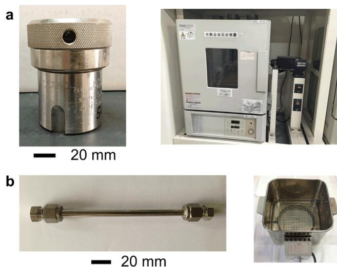
**Fig. 1.** Photographs of the reactors as well as the heating tools used for the synthesis of silicalite-1. a, The Teflon<sup>®</sup>-lined autoclave (left) and the air-circulating oven (right). b, The tubular reactor (left) and the pre-heated oil bath (right).
