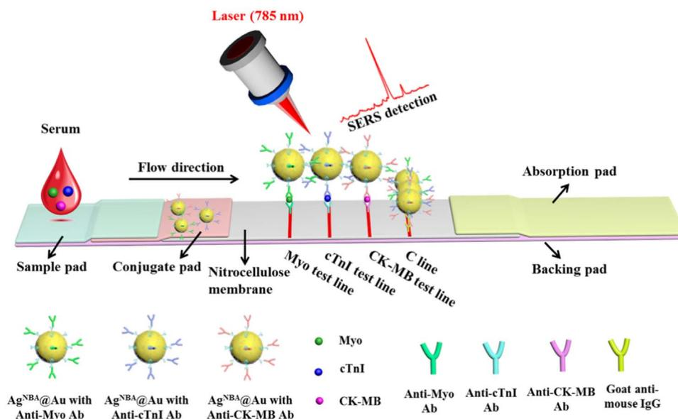
Fig. 1. Schematic illustration of the core-shell SERS nanotag-based multiplex LFA.
