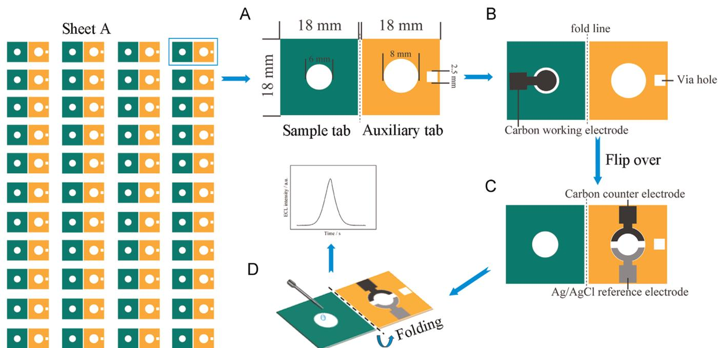
**Scheme 1.** Schematic representation of the fabrication and assay procedure of this origami device. Paper sheets were first patterned in bulk using a wax printer (sheet A). (A) One 3D origami device without the screen-printed electrodes. (B, C) Then electrodes were screen-printed on sheet A in bulk. Finally, sheet A was cut into individual 3D origami device. (D) After modification, the device was used to detect IgG.
