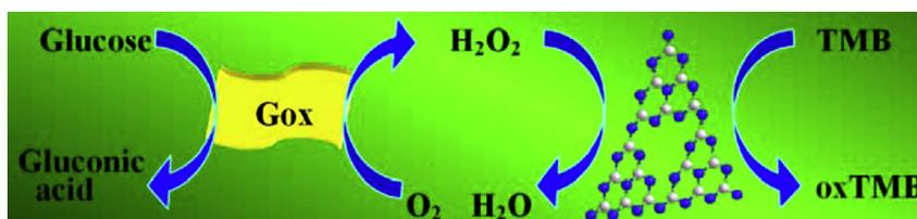
**Scheme 1.** Schematic illustration of colorimetric detection of glucose by using glucose oxidase (GOx) and  $g\text{-C}_3\text{N}_4$  peroxidase-like catalytic reactions.
