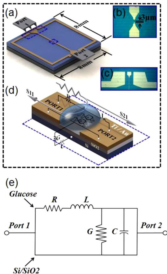
**Fig. 1.** Schematic diagrams of (a) GSG electrode for frequency based measurement. (b) The optical microscope image of detection area and (c) probing area. (d) The cross-sectional view of glucose detection region and (e) the equivalent circuit involving  $R$ ,  $L$ ,  $G$  and  $C$  in between two ports after glucose solution was dropped.
