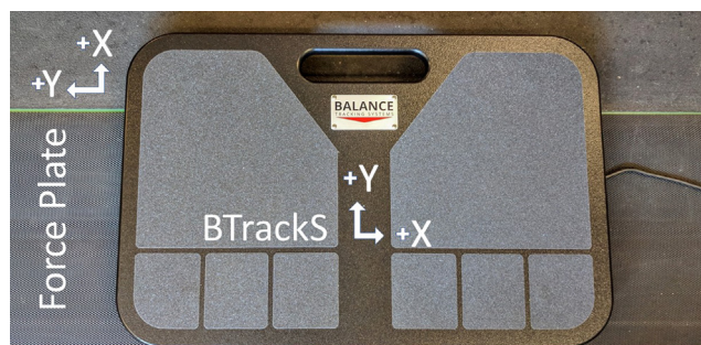
Fig. 1. Orientation of the BTrackS Balance Plate (atop the force plate) to the Bertec force plate. The directional difference was accounted for in the devised MATLAB script when calculating postural stability metrics.
