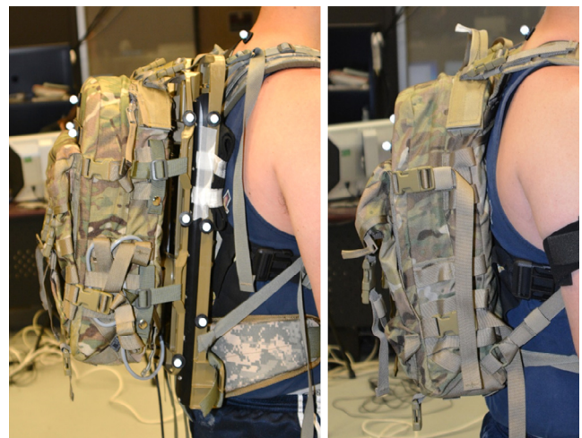
Fig. 1. Reflective markers were placed on the EHAP rigid and oscillating frame (left) to track vertical movement of the pack relative to the frame. Reflective markers were also placed on the face of the EHAP (left) and the standard assault pack (right).
