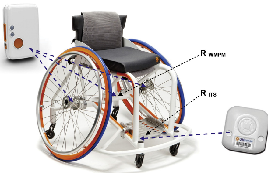
Fig. 1. Wheelchair measurement setup, with the Ubisense tag (ITS) mounted on the footplate and the Shimmer3 inertial sensors on frame and wheels. The reference point for the ITS ( R_{ITS} ) is the same as the tag, whereas the reference point for the WMPM ( R_{WMPM} ) is the frame centre. The WMPM2 reference point is in the middle of the footplate, so close to the R_{ITS} .
