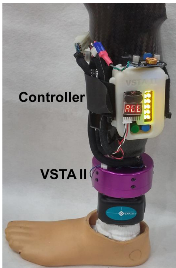
Fig. 1. VSTA II (purple) installed in pylon with control system attached to socket. (For interpretation of the references to color in this figure legend, the reader is referred to the web version of this article.)
