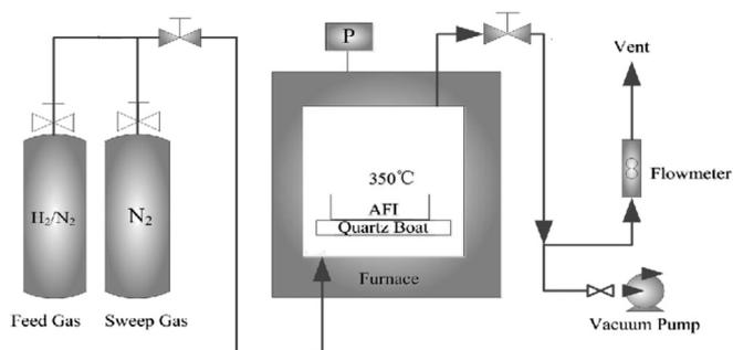
Fig. 1. Schematic diagram of the apparatus for SWNTs preparation via low-temperature hydrocracking.
