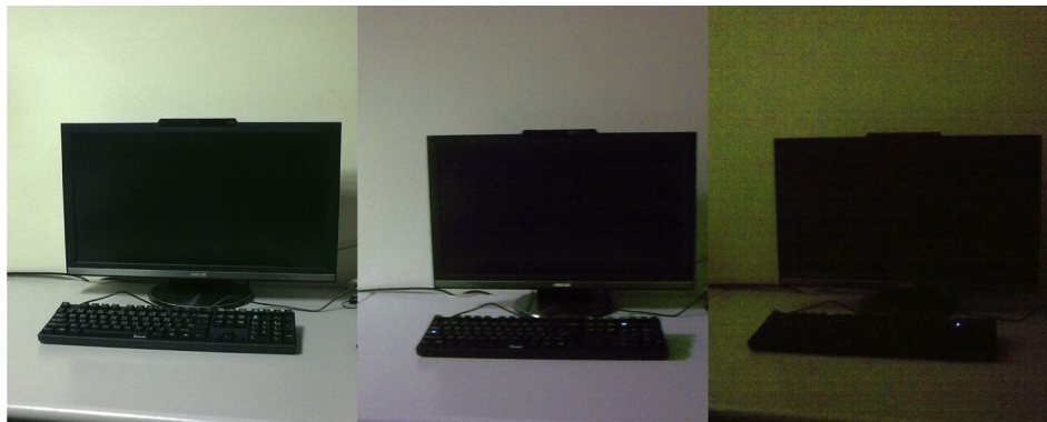
Fig. 1. Photographs of three levels of lighting in the test room as seen from where the participants sat. The left photo was the image under the high-brightness condition, the middle photo was the image under the medium-brightness condition, and the right photo was the image under the low-brightness condition.
