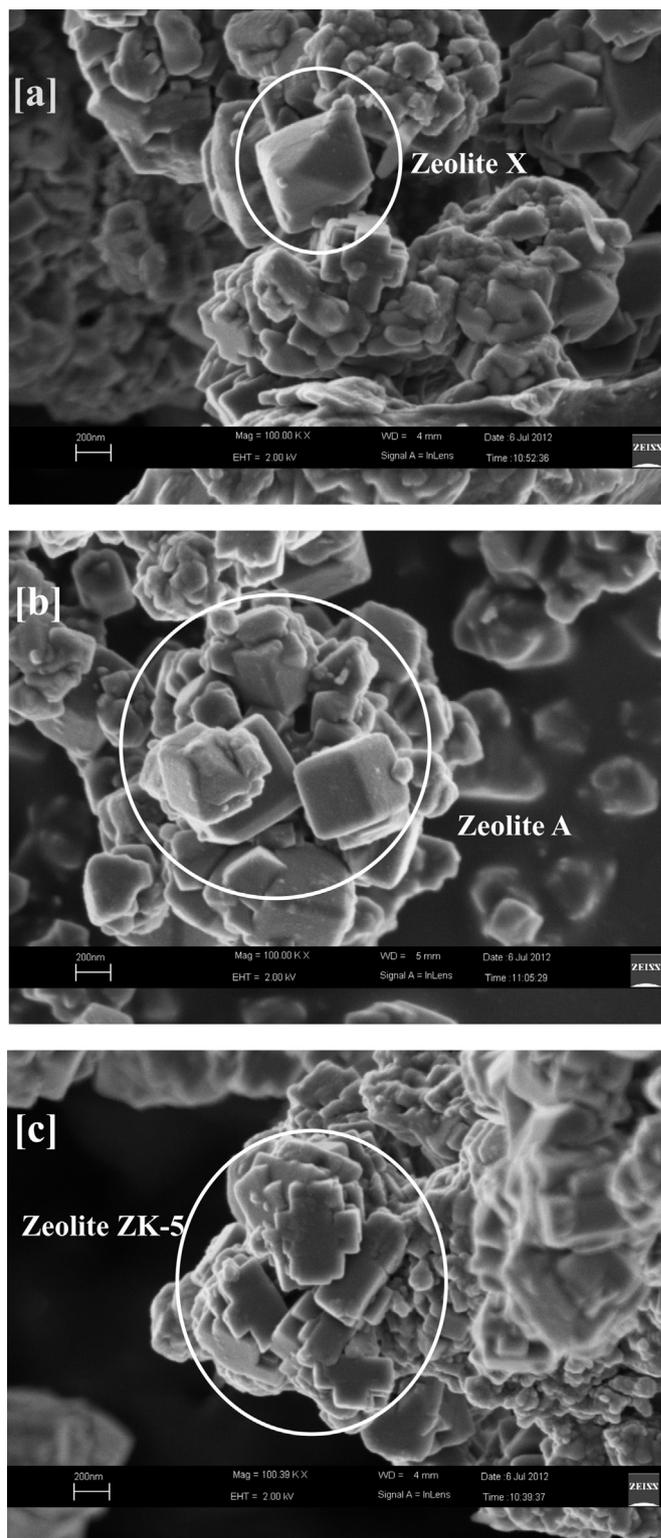
**Fig. 1.** Selected SEM images of zeolites synthesized using mixtures of fly ash and kaolinite after 48 h of incubation. [a] octahedral crystals of X-type zeolite (40FA sample); [b] cubic crystals of A-type zeolite (OFA sample); [c] typical morphology of zeolite ZK-5 (100FA sample).
