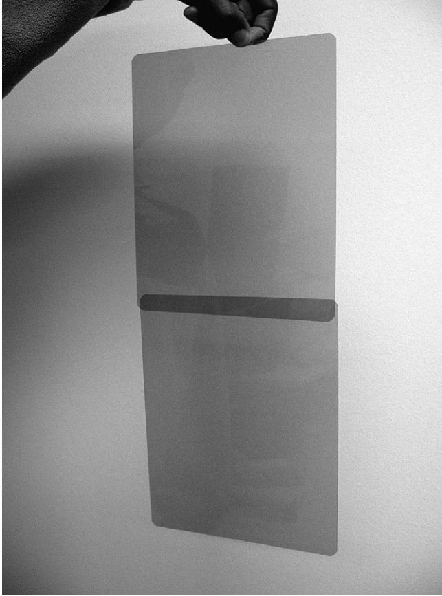
Fig. 1. Electrostatic charge causes sheets to stick. Each sheet has a buried conducting layer.
