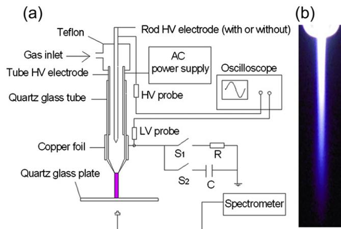
Fig. 1. Experimental setup of the device (a) and discharge photograph at peak applied voltage of 6.2 kV and Ar flow rate of 1 lpm with the rod-tube high voltage electrode (b).
