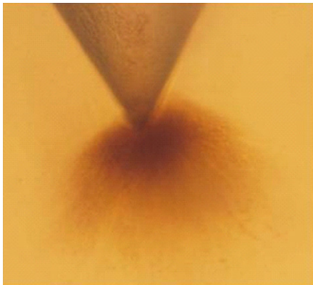
Fig. 1. Vented tree developed in low-density polyethylene.
