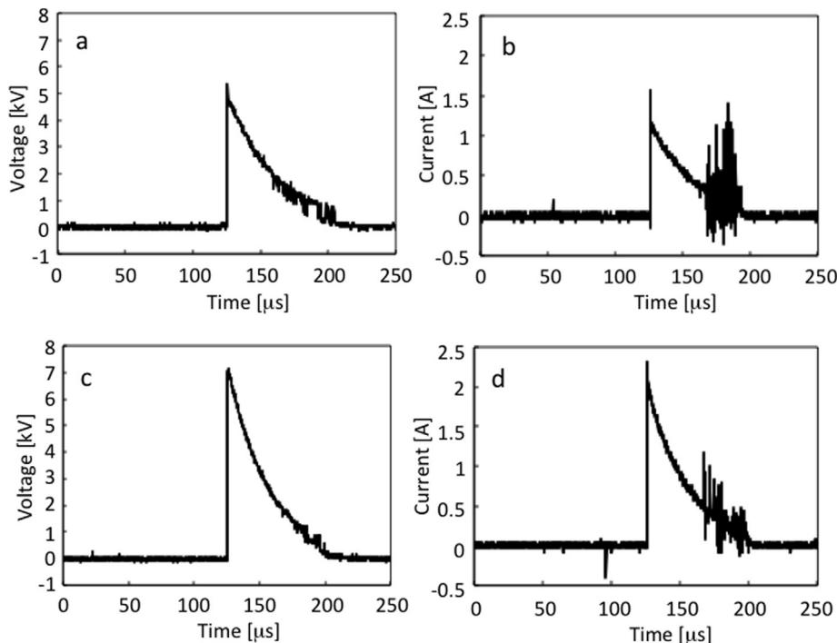
Fig. 1. The applied pulse voltage waveforms at 5 (a) and 7 kV(c), and the corresponding discharge current waveforms at 5 (b) and 7 kV (d).
