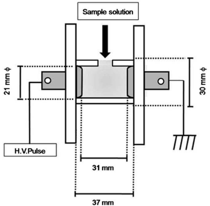
Fig. 2. Schematic illustration of PEF reactor used in this study.
