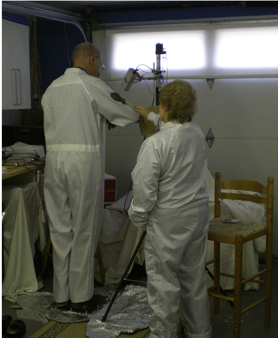
Fig. 1. Set-up for testing inhabited garments. Test subject standing on charge measurement plate with arm supported on insulated support. Test operator ready to tribocharge area of sleeve directly in front of JCI 140 Static Monitor.
