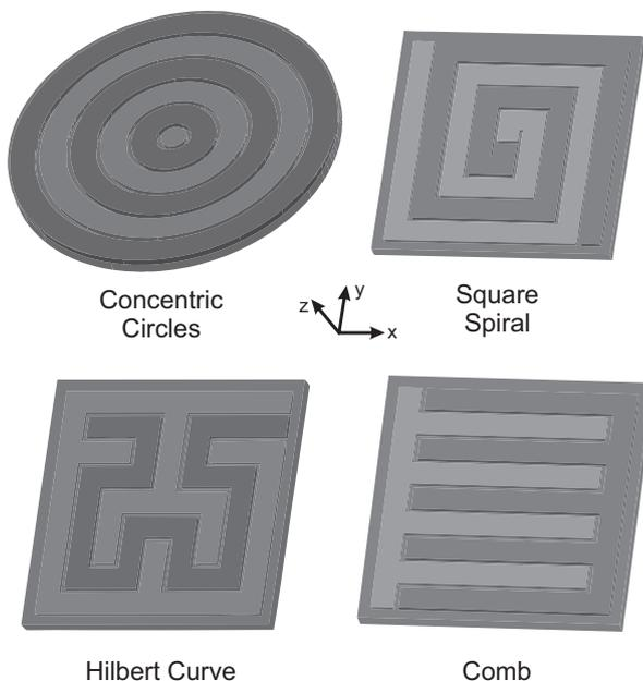
Fig. 2. Simulation models of different electrode patterns.
