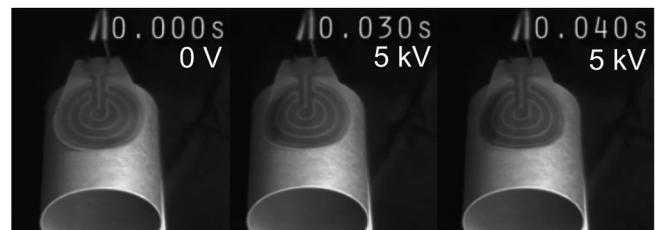
Fig. 3. High speed camera images of the conformal electrostatic adhesive adhering to a 65 mm diameter cardboard tube.
