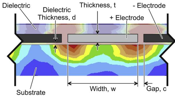
Fig. 1. Cross-section of an electrostatic adhesive pad.
