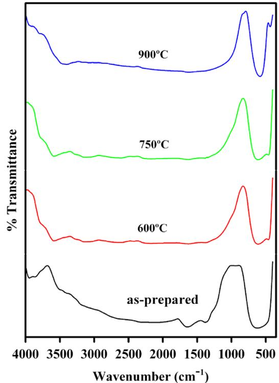
Fig. 2. FT-IR spectrum of Co-Zn  $\text{Fe}_2\text{O}_4$  nanoparticles.
