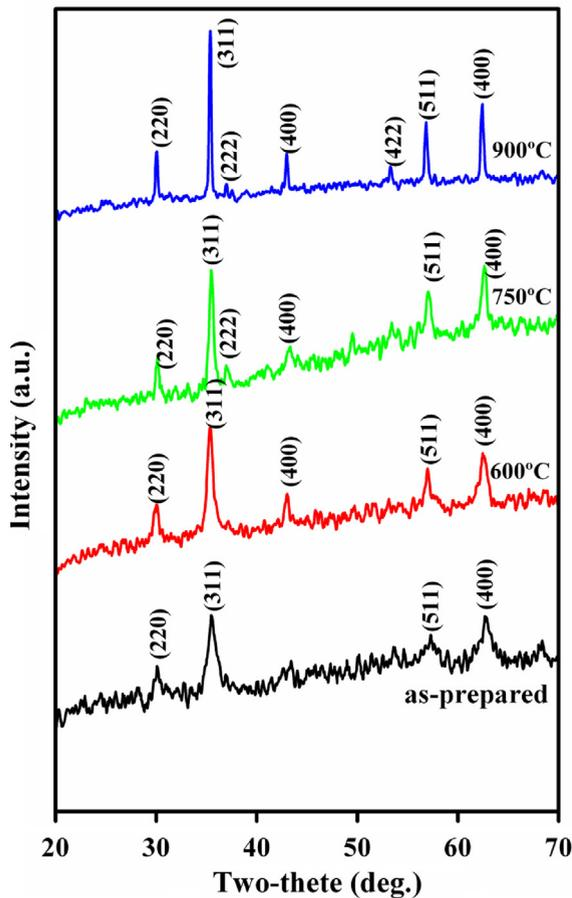
Fig. 1. Indexed XRD pattern of Co-Zn  $\text{Fe}_2\text{O}_4$  nanoparticles.
