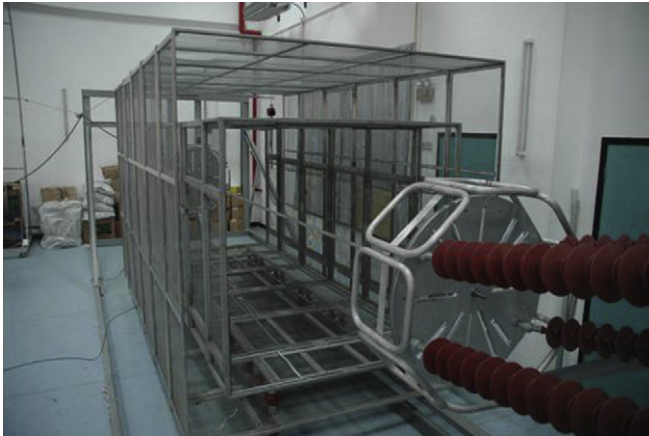
Fig. 1. General views of the corona cage used in the experiment.
