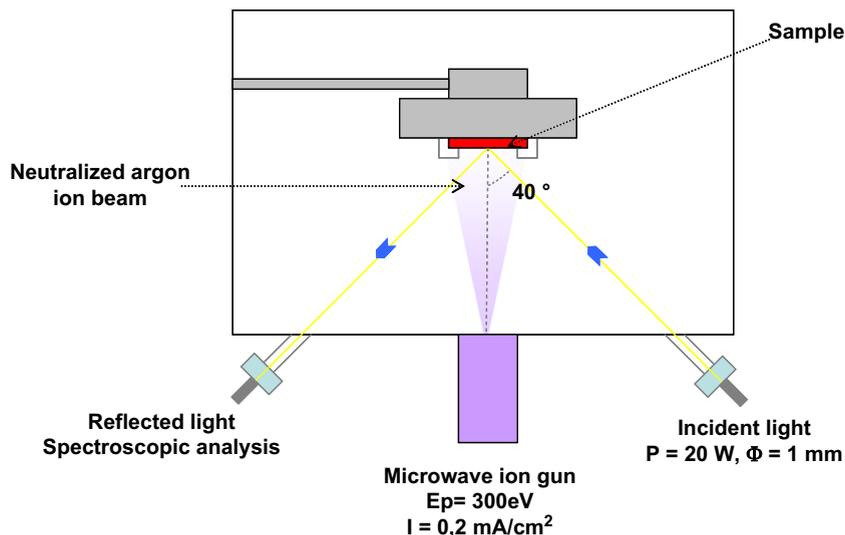
Fig. 1. Schematic view of the etching tool equipped with the spectroscopic reflectance.
