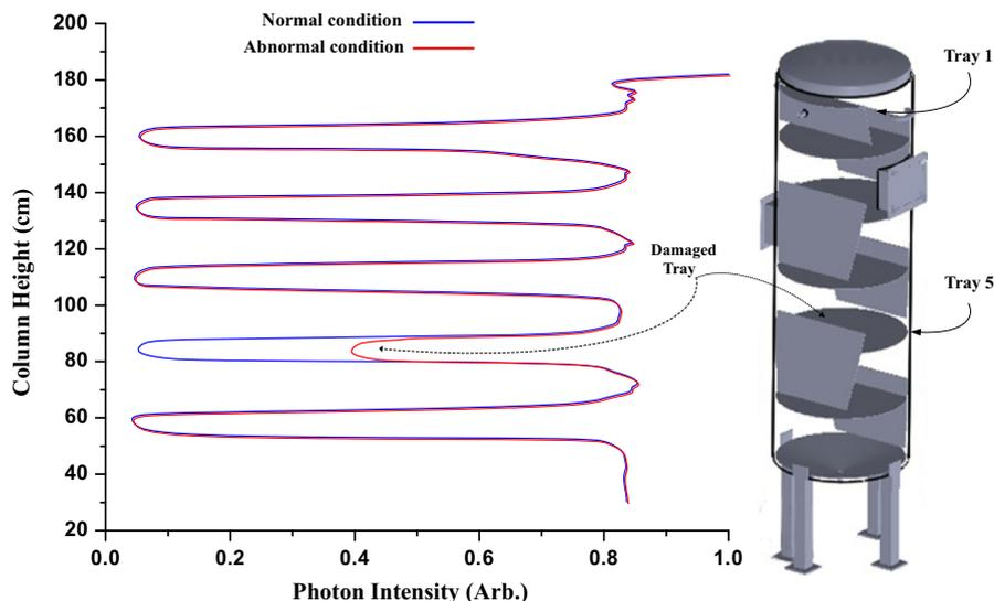
Fig. 1. Density profiles in normal and abnormal operation condition for typical Lab-scale distillation column.
