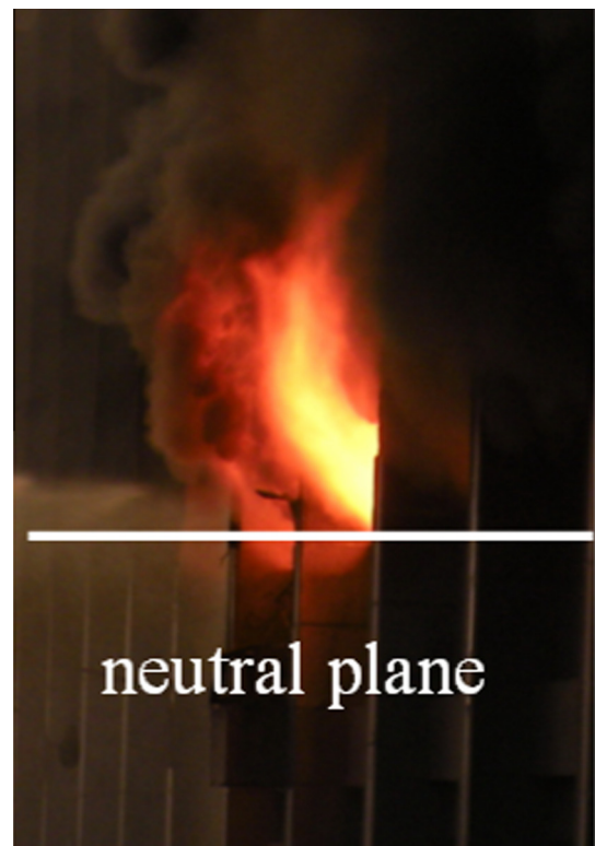
Fig. 2. Neutral plane in the real fire.
