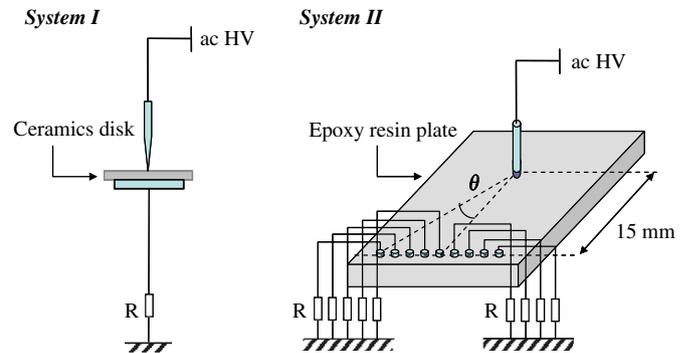
Fig. 1. Electrode systems used for the study of the discharge propagation parameters (system I) and for the analysis of the current and chemical products distributions on the dielectric surface (system II).
