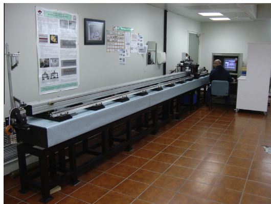
Fig. 1. General view of UME motorized 5 m tape comparator.
