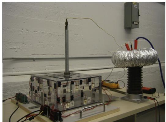
Fig. 2. Set-up, a PMMA case with HTUTs mounted above.
