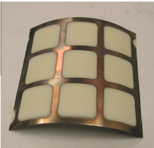
Fig. 1. Piezoelectric HTUT sensors.
