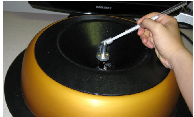
Fig. 2. Magnetic levitation haptic device (right hand operation).
