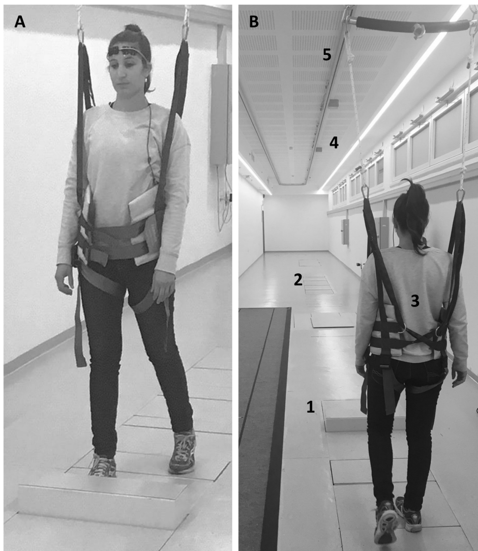
Fig. 1. The setting of the obstacle course testing. (A) the location of the fNIRS probes on the forehead (without the black fabric that cover the probes) and front view of the harness. (B) the obstacle course area: 1-anticipated obstacle module, 2-unanticipated obstacle module, 3-safety harness, 4-location sensor, 5-elliptical rail that was used to support the safety harness.
