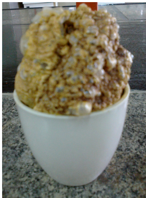
Fig. 2. The xerogel of TEN sample.
