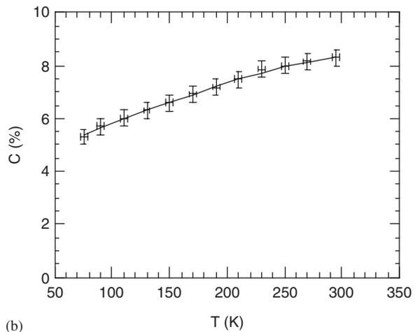
Fig. 1. (a) EBIC image at 300 K of the  $p/p^+$  sample. (b) Curve of the EBIC contrast at the oxygen precipitates as a function of temperature in the 77–300 K range in the same sample.
