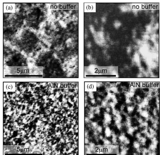
Fig. 1. (a) SCM images of (a) and (b) HFET structure with no AlN buffer layer, exhibiting dislocations at nucleation island domain boundaries, and (c) and (d) HFET structure with a  $\sim 60$  nm AlN buffer, exhibiting randomly distributed dislocations.
