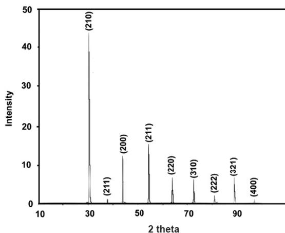
Fig. 1. XRD pattern (Cu $K\alpha$  irradiation) of  $BaSnO_{3-\delta}$  synthesized in evacuated silica tube.
