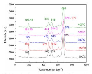
**Fig. 1.** Raman intensity as a function of wave number before annealing for cobalt oxide samples grown at different temperatures.
