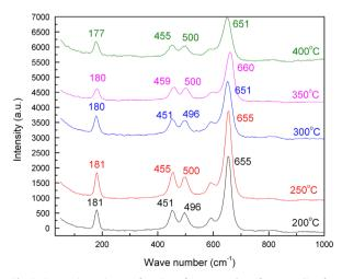
Fig. 2. Raman intensity as a function of wave number after annealing for cobalt oxide samples grown at different temperatures.
