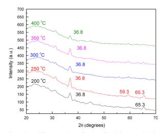
**Fig. 4.** X-ray diffraction peaks as function of  $2\theta$  before annealing for cobalt oxide samples grown at different temperatures.
