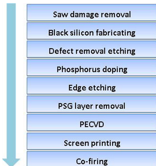
Fig. 1. The procedure of fabricating multicrystalline black silicon solar cell with nine steps.
