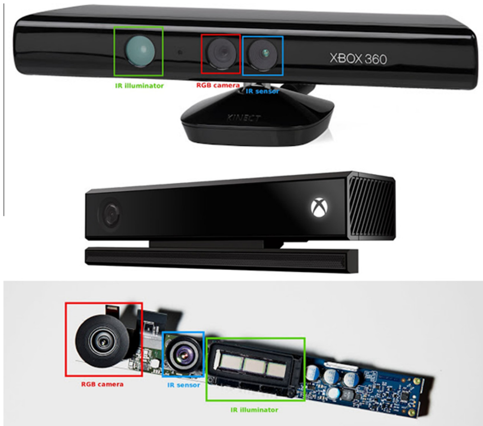
Fig. 1. Kinect I laser scanner with highlighting of IR illuminator, RGB camera and IR sensor (top), and Kinect II laser scanner with RGB camera, IR sensor and IR illuminator (bottom).
