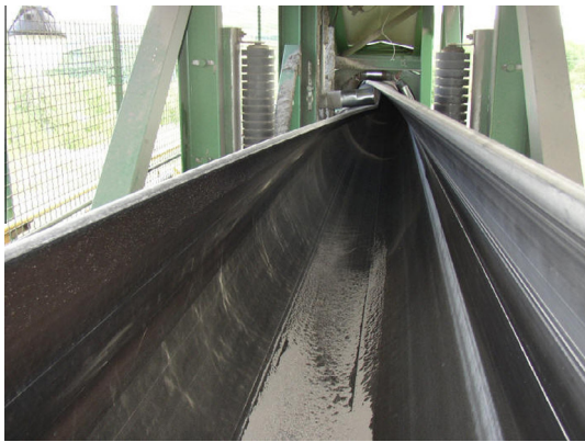
Fig. 1. Folding belt from flat shape into a pipe shape. Image Courtesy of Specialty Welding & Fabricating of New York, Inc.
