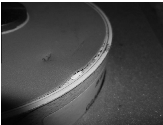
Fig. 2. Photograph of a force transducer in which the seal was accidentally broken.
