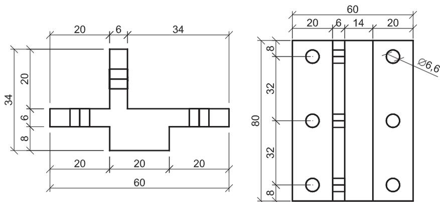
Fig. 2. Detailed view of the connecting element.
