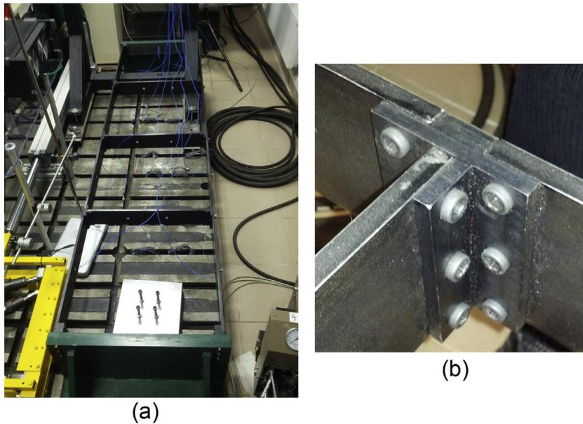
Fig. 1. View of the tested frame and the connecting element.
